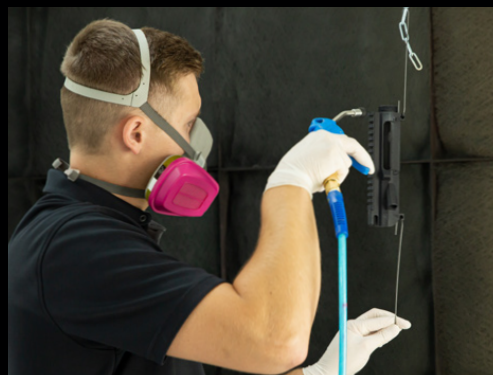
Before spraying, blow off all your parts.
